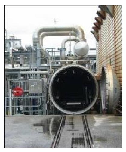
Wood is heated to ca. 165°C in aqueous environment at superatmospheric pressure.
