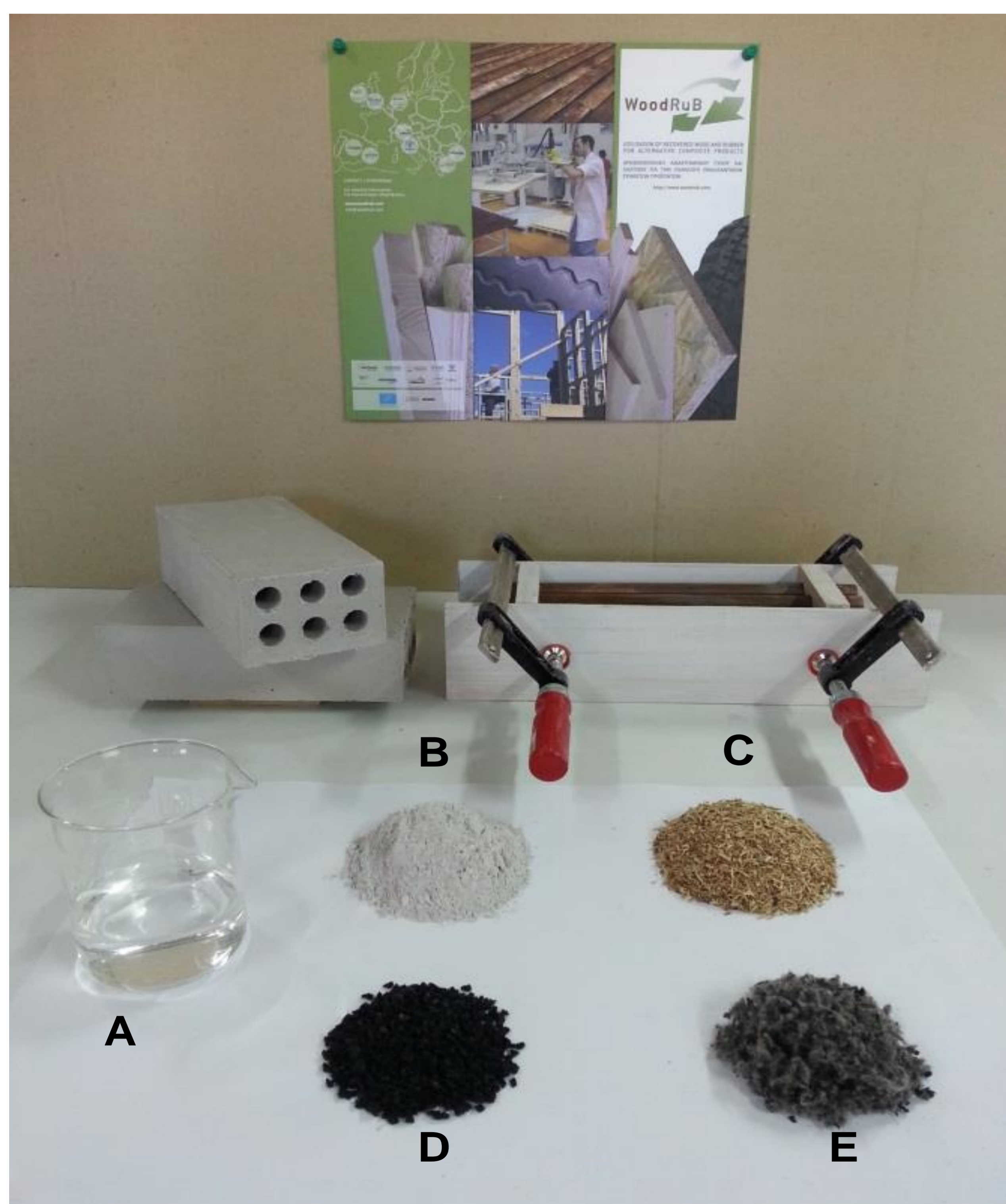
Figure 1. . Water (A), gypsum (B), recovered wood (C) and rubber fractions (D), and reinforcement material (E) for the manufacturing of WoodRub BRICKS (up left) by using simple moulds (up right)
