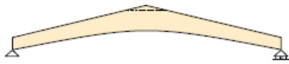
Bent ridge beam
