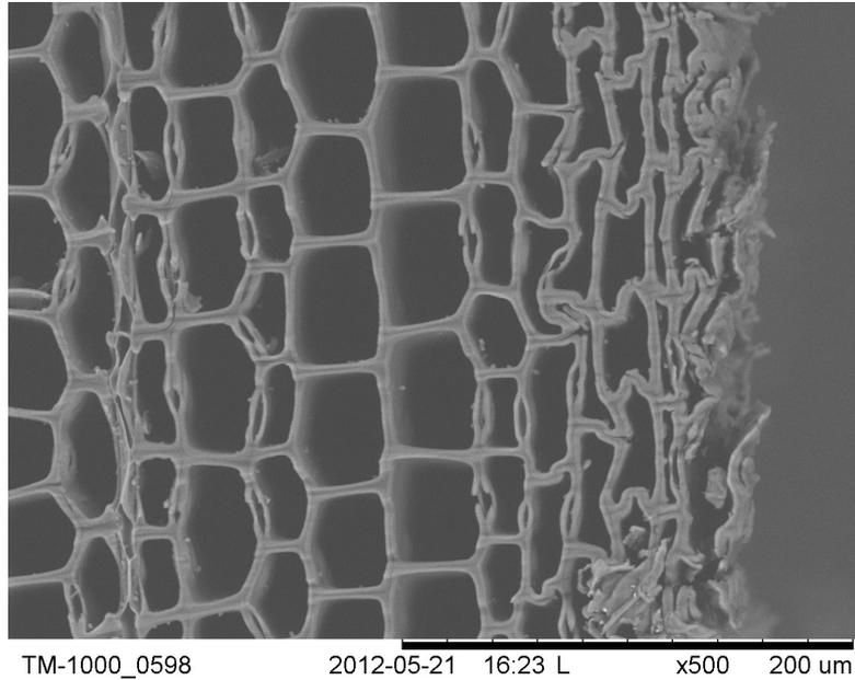
**Figure 1: SEM image of laser ablated control sample (outer edge to right of image)**
