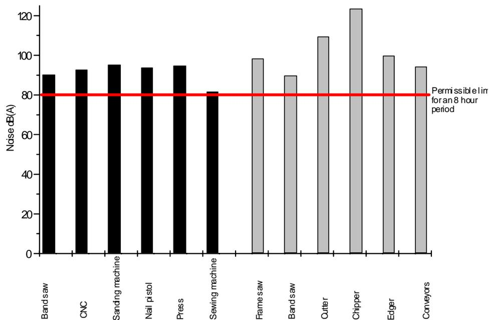
**Figure 1. Noise levels which are emitted by the most important machines in furniture (shown in black) and wood (shown in grey) processing industries.**
