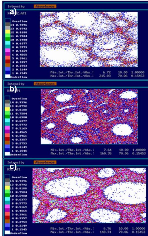
Figure 1: UV microspectrophotometric scanning profiles of the untreated control (a), koto treated with 10% (b) and 30% MMF resin (c).
