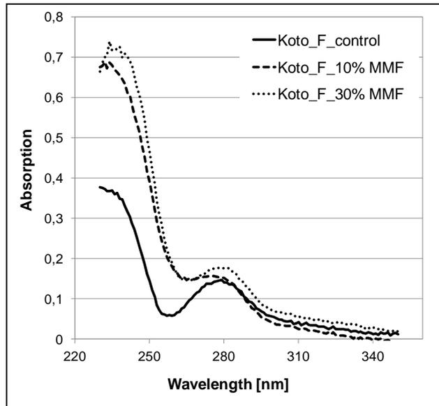
Figure 2: UV absorption from UMSP point measurements.
