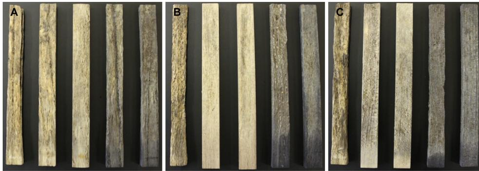
**Fig. 4.** Photos of unmodified and NMM or NMM-BS modified ash (A), beech (B), and maple (C) wood stakes after 32 weeks of exposure in soil according to ENv 807. In every photo, the stakes from left to right are: unmodified control, 10% NMM, 20% NMM, 10% NMM + BS, 20% NMM + BS.
