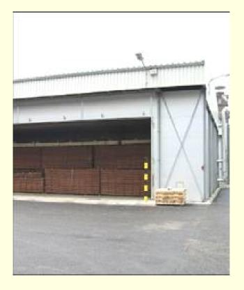
Restore the moisture content from 1% (after curing) into the more suitable 6-8% MC (necessary for manufacturing)
