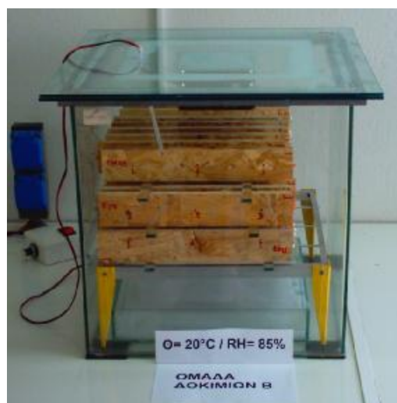
Figure 3. Conditioning chamber containing specimens
